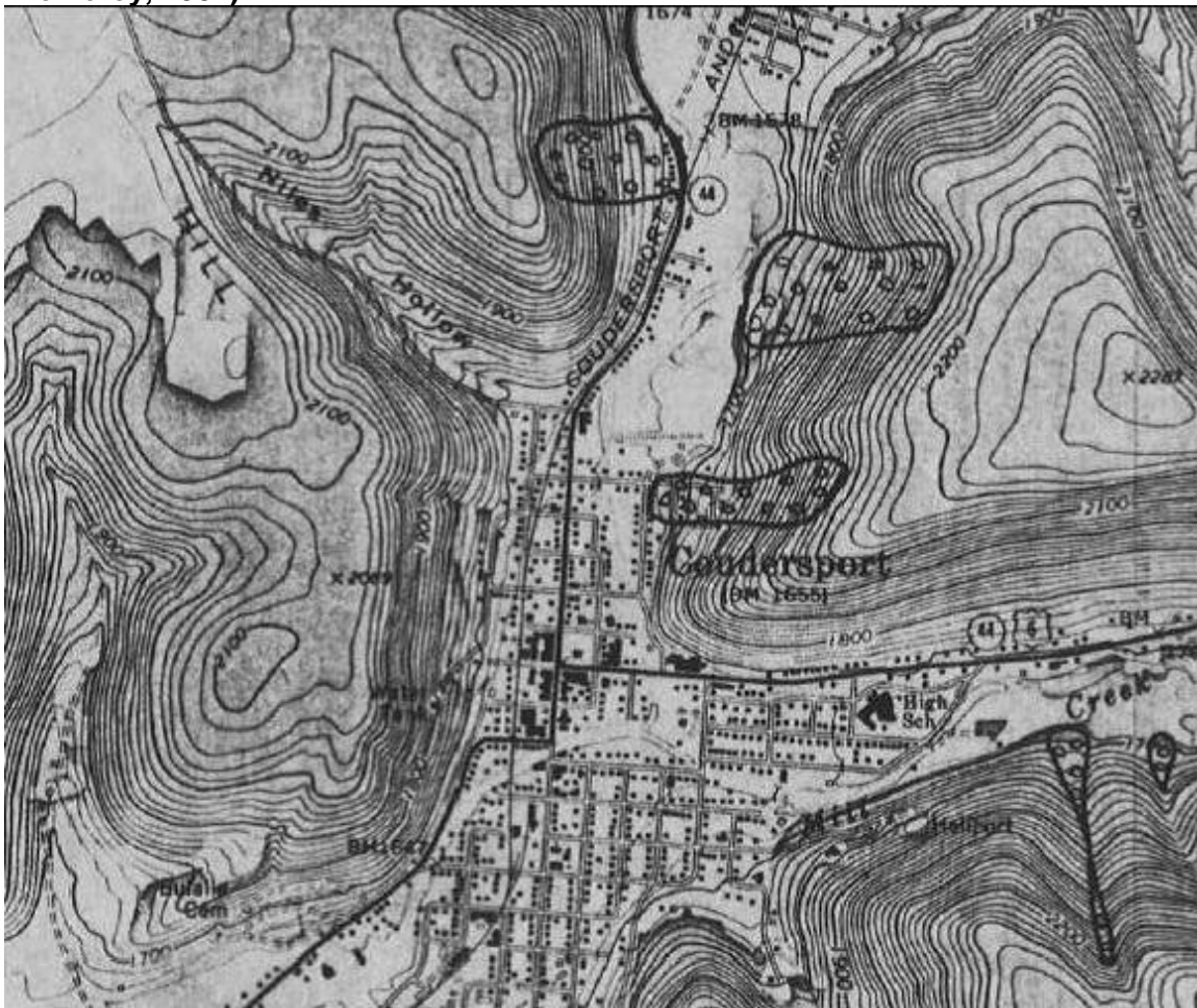
Figure 4.4.7.3-1 Landslide inventory map for Coudersport, PA from USGS Open File Map 81-238 (G-16 by John S. Pomeroy, 1981).
