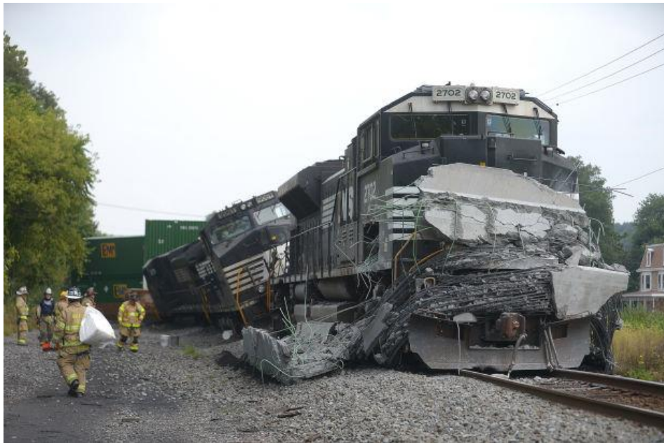
Figure 4.3.15-5: A freight train struck a tractor-trailer hauling a 135-foot-long concrete bridge span at the Brandtsville Crossing in Monroe Township, Cumberland County, PA on September 12, 2013 (Photograph courtesy of The Sentinel , 2014).
